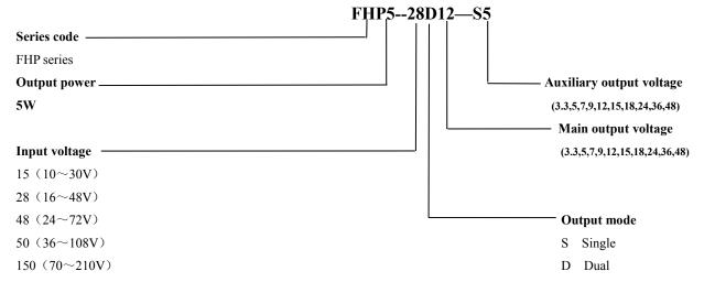
NOTE: "-" in model refers to isolation. It is always isolated between input and output. For this reason, the first "-" is necessary. If it is not isolated between main and auxiliary outputs, there is no the second "-". If there is no auxiliary output, there is no -SAOUT.
