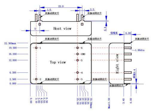
Note: 1. The tolerance of needle diameter and between two pins is  $\pm 0.1$ mm;
