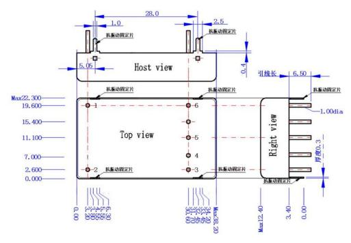
Note: 1. The tolerance of needle diameter and between two pins is  $\pm 0.1$ mm;
